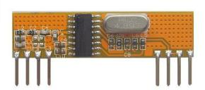
315/433.92Mhz in USA under FCC Part 15 regulation. The CY16 is base on a single-conversion, super-heterodyne receiver architecture and incorporates an entire Phase-Locked Loop (PLL) for precise local oscillator generation. It can be used in OOK/ HCS/ PWM modulation signal and demodulate to digital signal. CY16 have a high performance at a competitive cost and easily to design your product.
