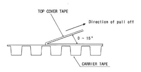
[Figure 1] Carrier Tape Dimensions
