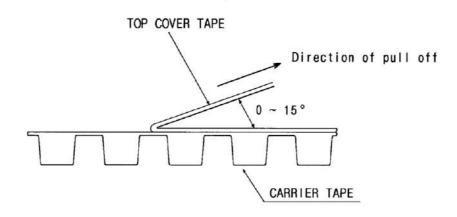
[Figure 1] Carrier Tape Dimensions
