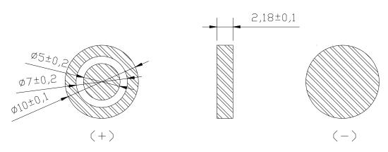
Electrode material: Ni with Au top layer. Electrode thickness: Au 0.1  $\mu$  m ~ 0.2  $\mu$  m; Ni 1.5  $\mu$  m ~ 2.5  $\mu$  m.
